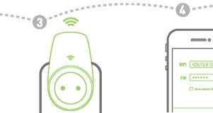
Plug NEO Switch into a power outlet, then press ON/OFF button for 5 seconds and release it. The Wi-Fi indicator light will flash quickly. NEO Switch is now ready for synchronization.
